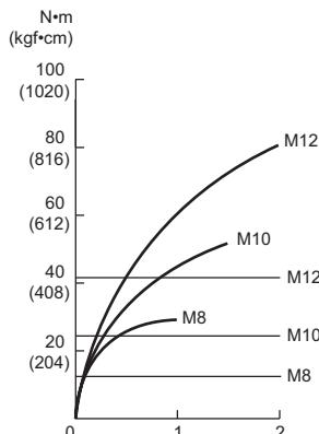
1. Fastening time (second) 2. Fastening torque
